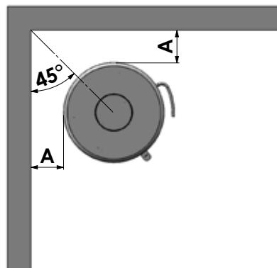
We recommend that the stove be installed at least 10 - 15 cm from masonry, in order to allow heat to circulate and to facilitate the cleaning of the inside and outside of the stove. A layer of wallpaper on a brick wall is normally viewed as non-flammable material.
