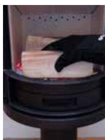
The stove door must be opened gently the first 2 - 3 centimetres, then you should wait until the pressure has equalised before opening the door all the way. This technique will prevent smoke from getting out, particularly when there is a poor draught.
